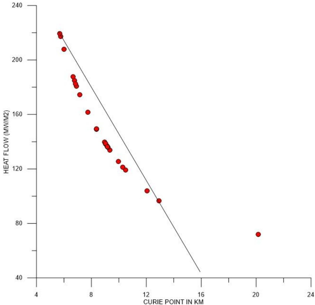
Figure 3.11. Relationship between Curie Depth and Heat Flow within the Study Area
