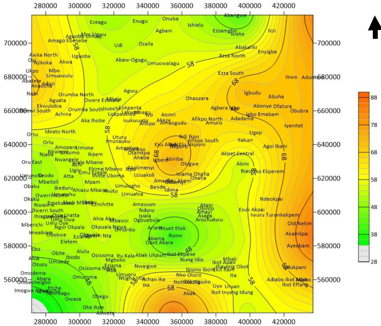
Figure 3.9. Geothermal Gradient Map of the Study Area
